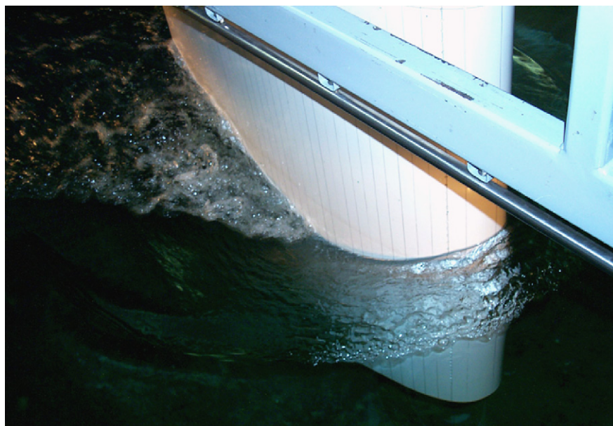
Fig. 1. Surface-piercing NACA24 foil at Fr = 0.37 .
