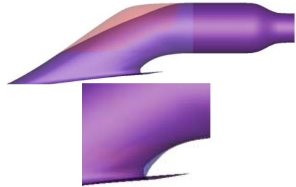
Fig. 9. Selected initial DC waterjet duct geometries for morphing
